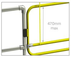
**9.** Ensure mid rail is level, and gap between top of gate and mid rail is not greater than 470mm, and torque clamps to 19 Nm.
